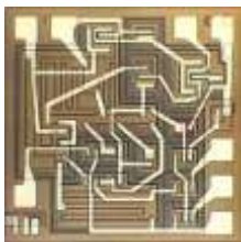
Talbert and Widlar's \mu A709 high-performance operational amplifier (1965)
