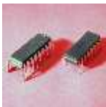
Don Forbes, Rex Rice, and Bryant ("Buck") Rogers developed the DIL package (1965), before mainly "TO" (transistor outline) formed as metal cans where used
