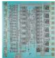
Micromosaic - standard cell design for GE Avionics (1968)
