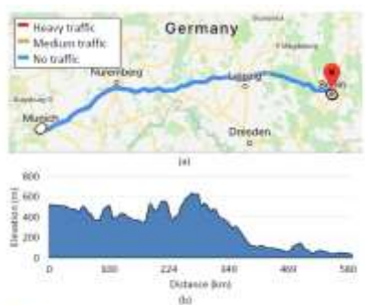
Figure 5. Example of driving route: (a) road traffic information and (b) road slope information.
